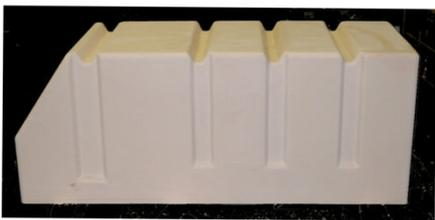
Example of a HYTAC-LP plug in the finished shape for use in thermoforming a full size freezer liner.
