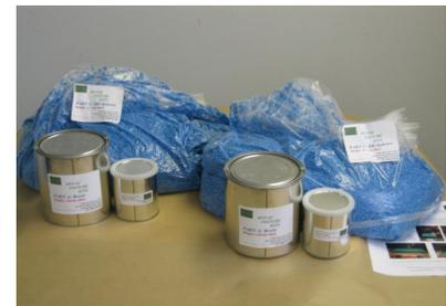
HYVAC is supplied in a 0.5 ft<sup>3</sup> kit, conveniently separated into two distinct 0.25 ft<sup>3</sup> mixtures. (0.25 ft<sup>3</sup> is approximately 1.9 gallons.)
